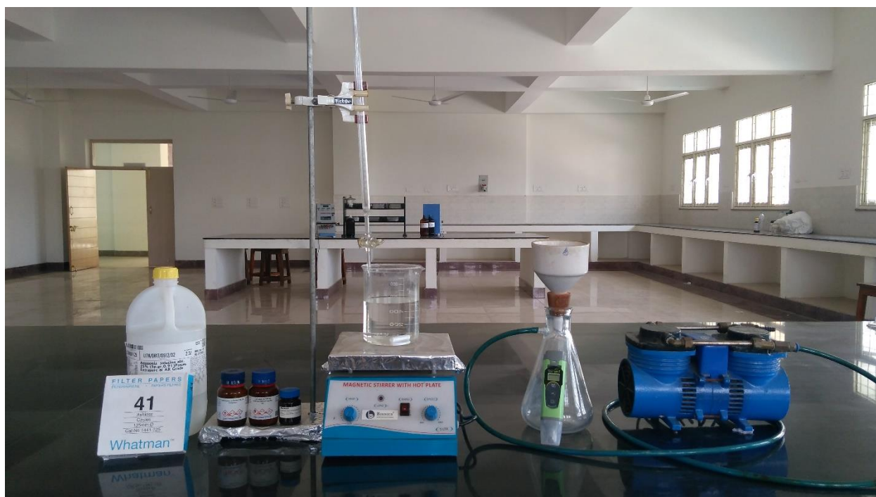
Fig. 3.2: Experimental setup used for the co-precipitation process.
