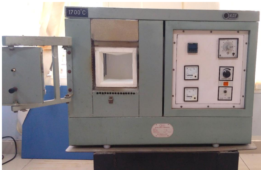
Fig. 3.4: Box type electric resistance furnace used for sintering of compacted samples.
