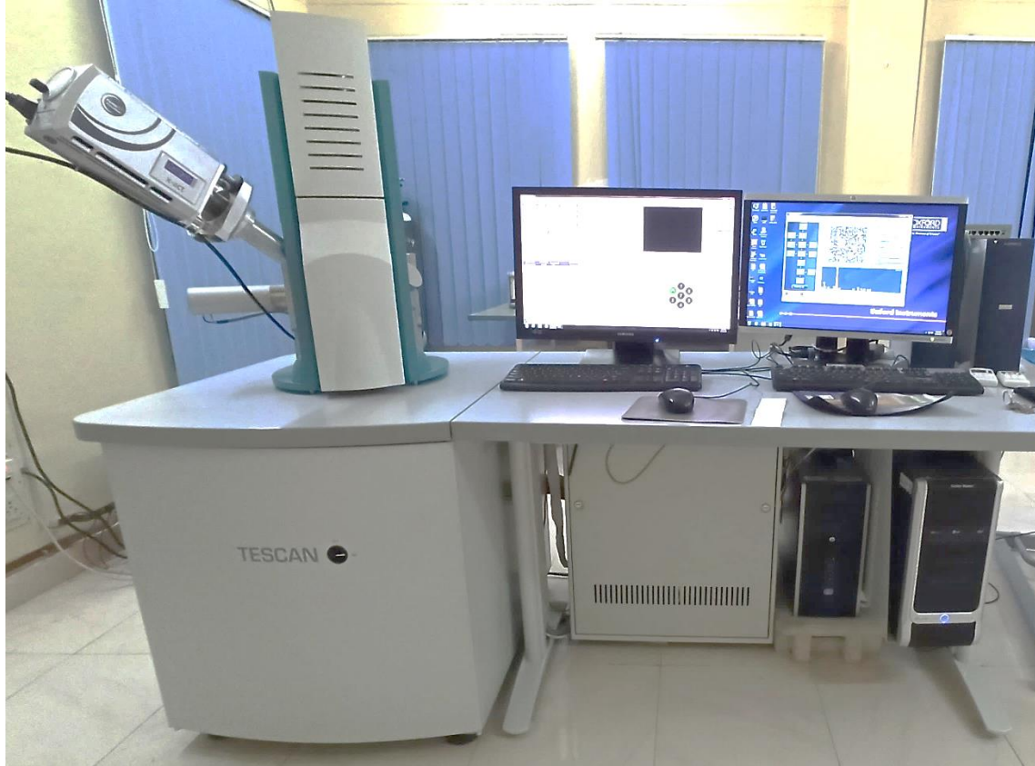
Fig. 3.9: Scanning Electron Microscope used for microstructural analysis of samples.
