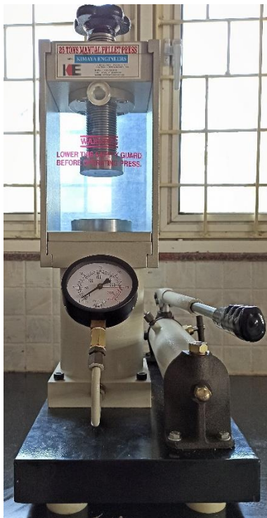
Fig. 3.3: Uniaxial hydraulic press used for compaction of powders.
