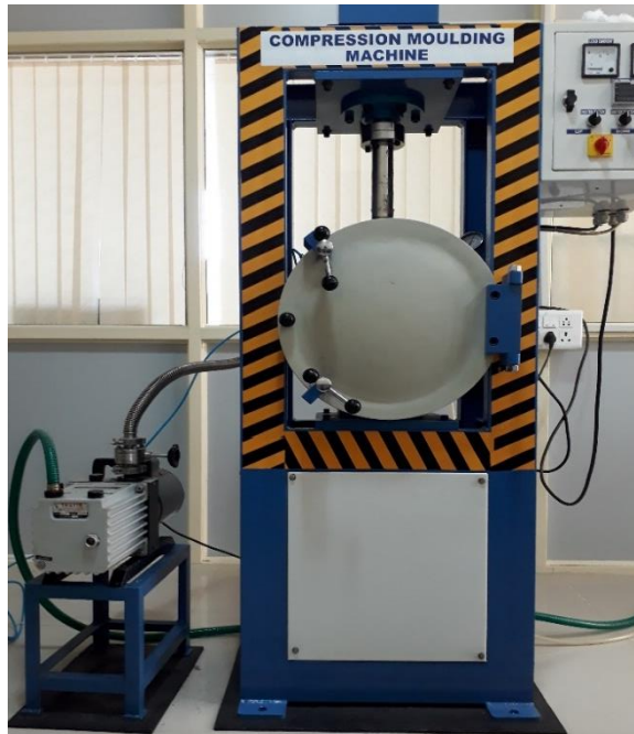
Fig. 3.3 Hot press equipment with vacuum pump arrangement
