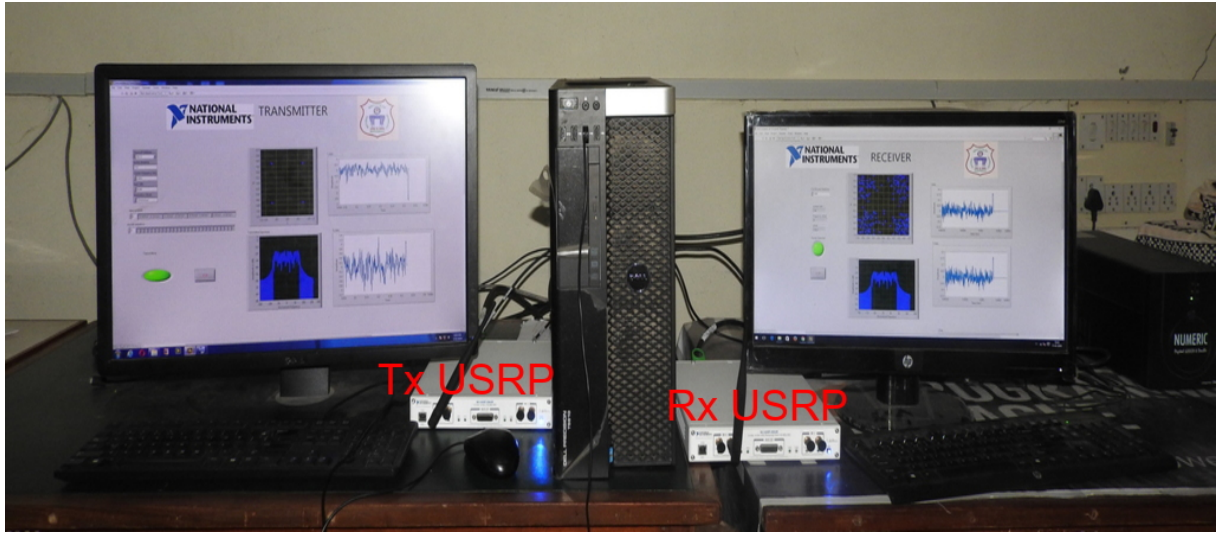
Figure 2.2: Experimental set-up used for testing algorithm in real time environment
