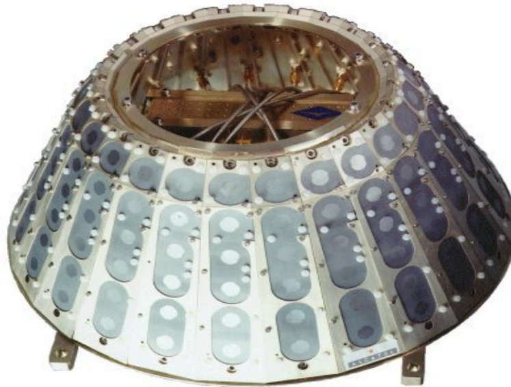
Figure 1.6 A conical conformal array for data communication from a satellite [13-14].
