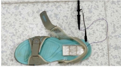
Fig. 8: Shoes with One Layer of PVDF Films
