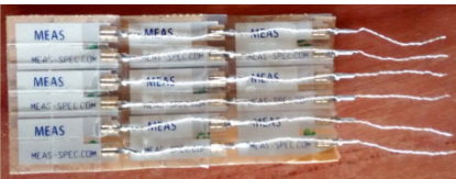
Fig. 3: One Layer Comprising of Nine Film Sensors
