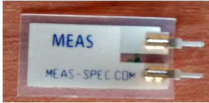
Fig. 2: PVDF Laminated Film Sensors-LDT0-028K/L w/crimps
