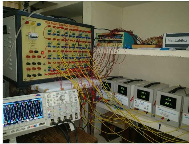
Fig. 7 Photograph of the experimental set-up for realising 13-level asymmetrical switched dc source inverter
