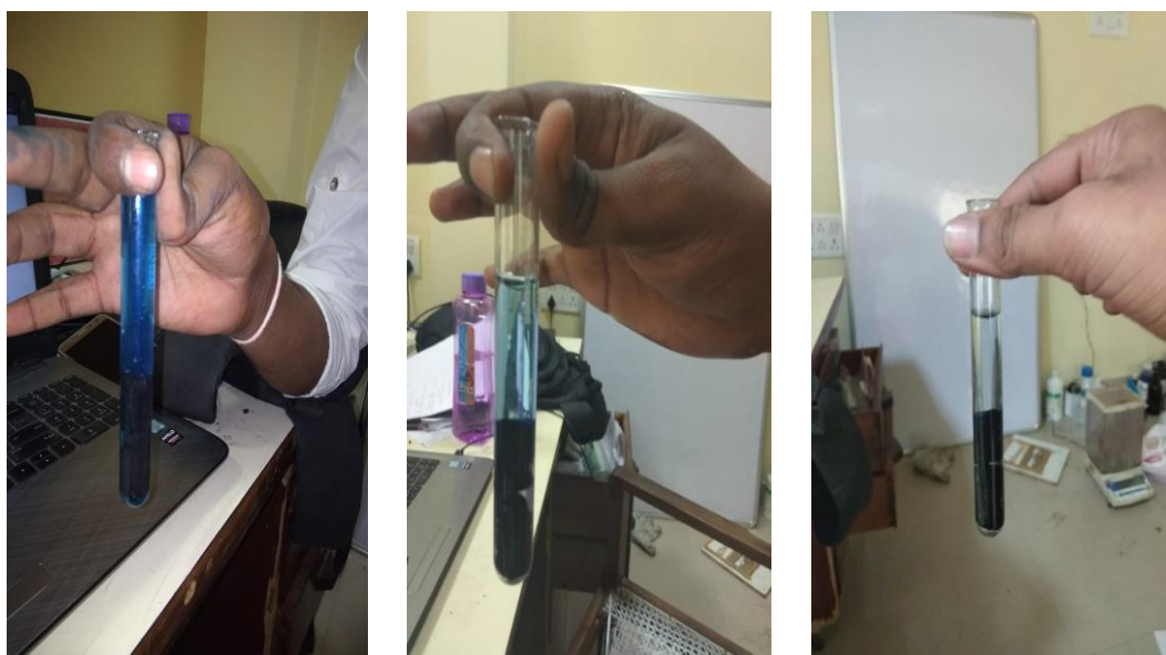
Figure 6.12 Methylene blue dye adsorption by composite filter
