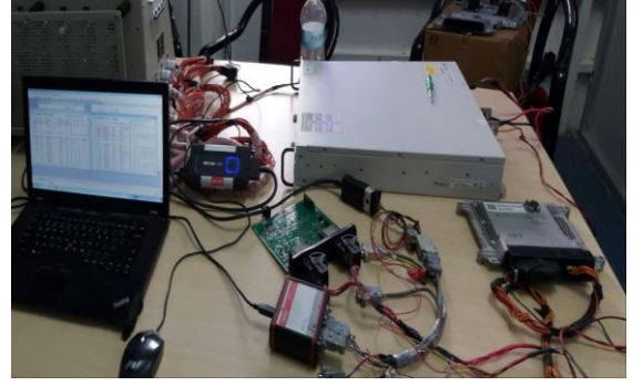
Fig. 3 Performance evaluation test setup for gateway ECU
