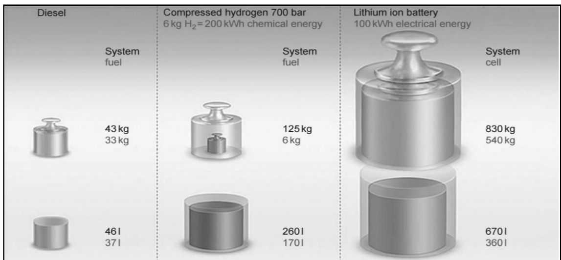
Figure 2.3 Energy Storage System weight and volumes for various energy carriers [63]
