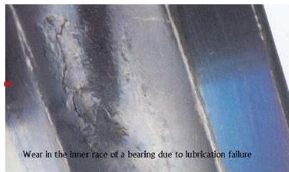
Fig. 1.14. Lubrication failure of bearing [28]
