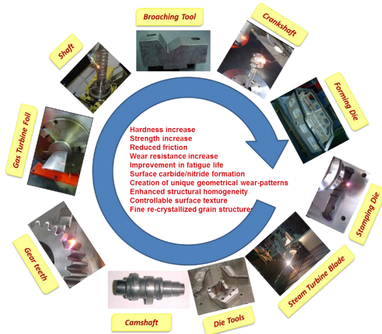
Fig. 1.18. Typical industrial applications employing laser surface hardening process
