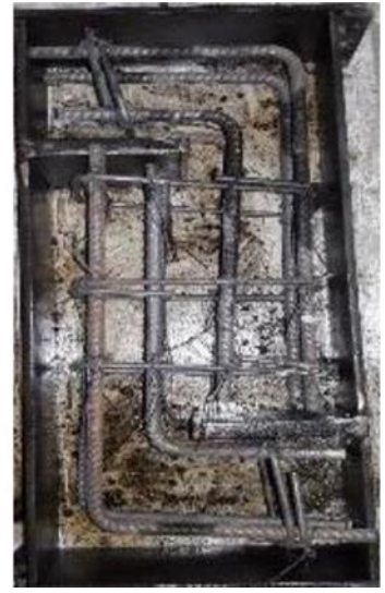
Push-off specimen with reinforcement before casting
