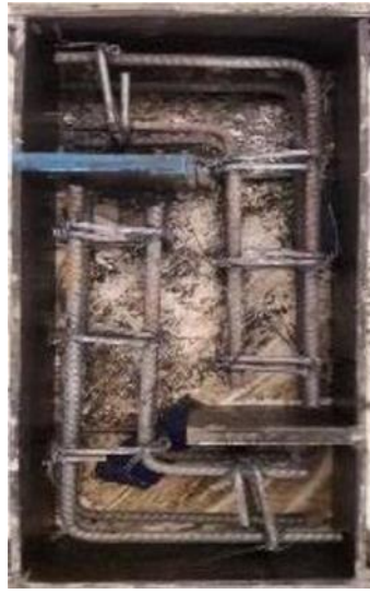
Push-off specimen with reinforcement before casting
