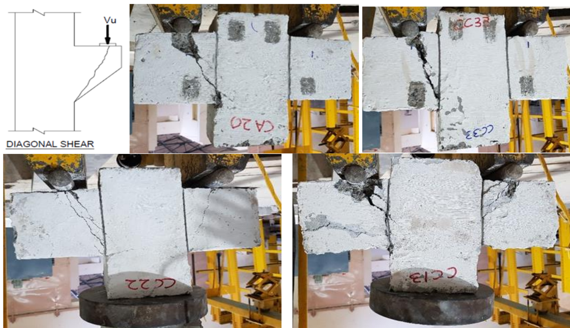
Figure 6.10: Failure pattern of corbel/bracket
