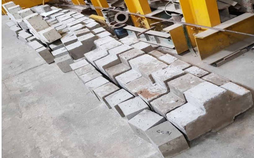
Figure 6.7: Cast specimens left for outdoor curing
