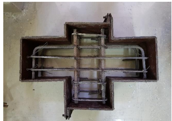
Corbel specimen with reinforcement
