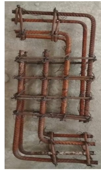
Push-off specimen with reinforcement before casting
