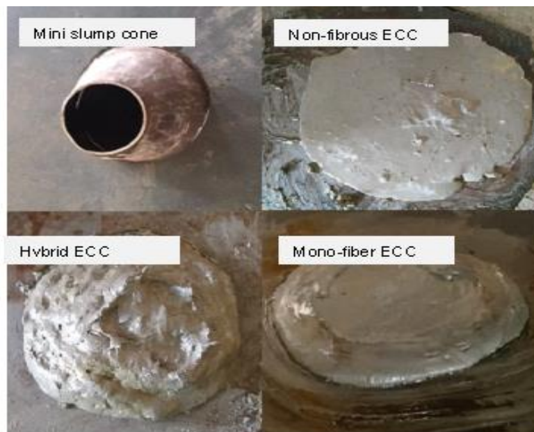
Figure 6.1 Typical view of mini slump cone test
