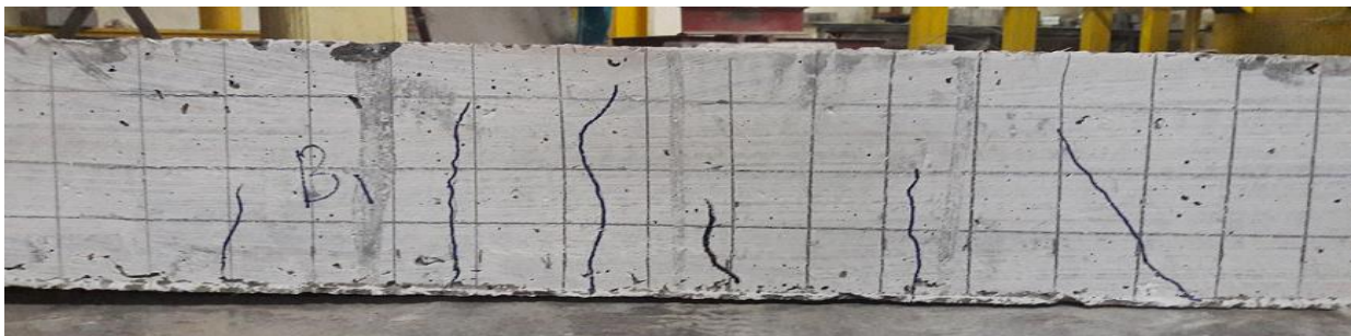
5.8 (a) Control RC beam after complete failure
