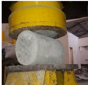
Figure 4.12 Split tensile strength test setup
