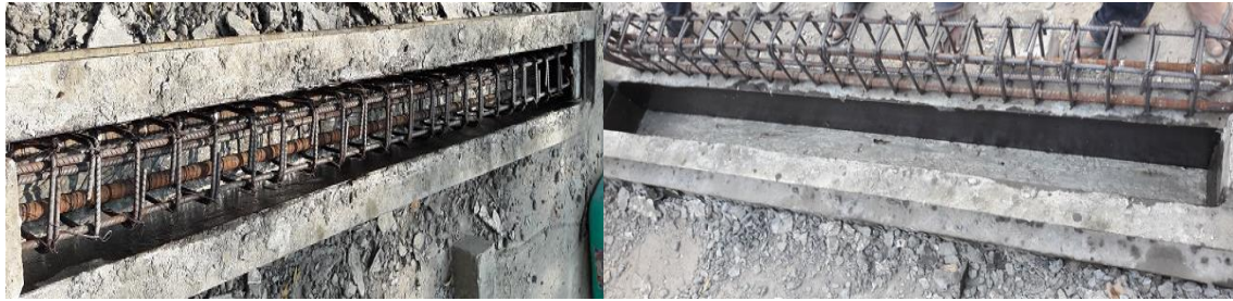
4.9 (a) Reinforcement cage in the mould
