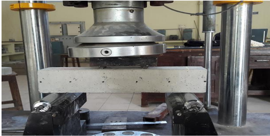
Figure 4.13 Flexural strength test setup
