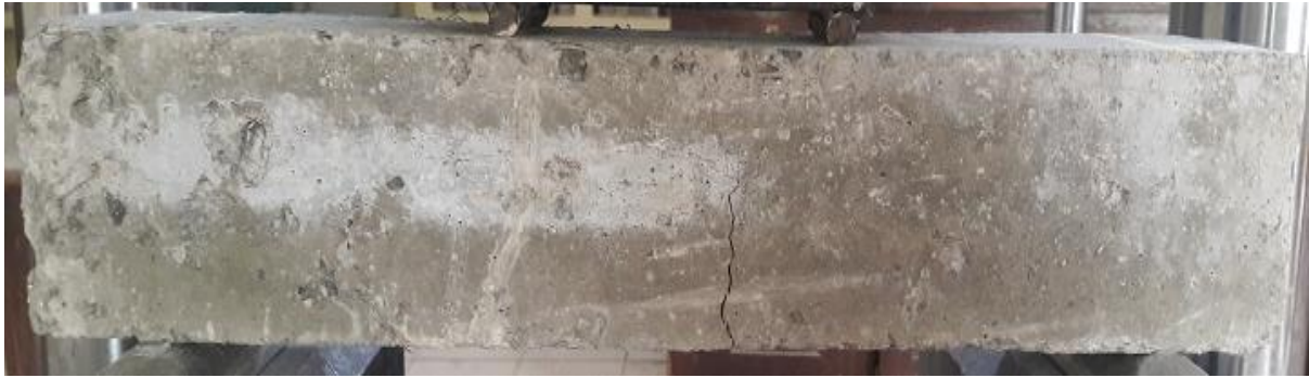
Figure 5.4 Flexural failure of SFRC specimen
