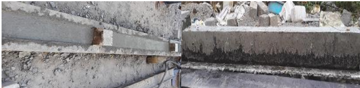
4.9 (c) Finished FGRC beam surface
