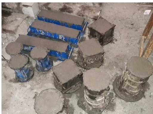
4.4 (c) Casting of specimens
