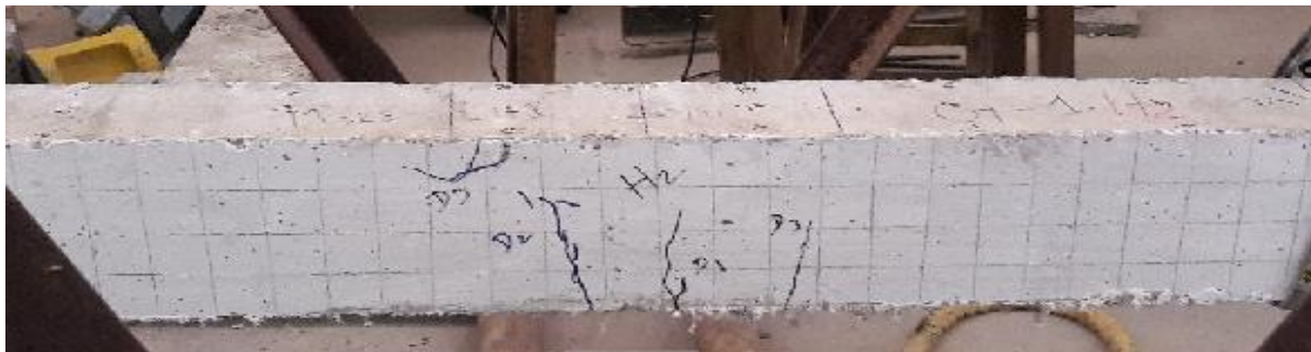
6.8 (b) FGRC beam with one layer of ECC material after complete failure
