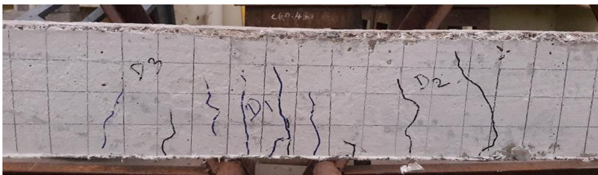
5.8 (c) PPFRF beam after complete failure
