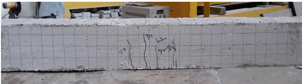
6.8 (d) FGRC beam with three layers of ECC material after complete failure
