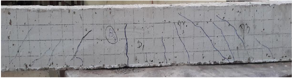
6.8 (a) Control RC beam after complete failure
