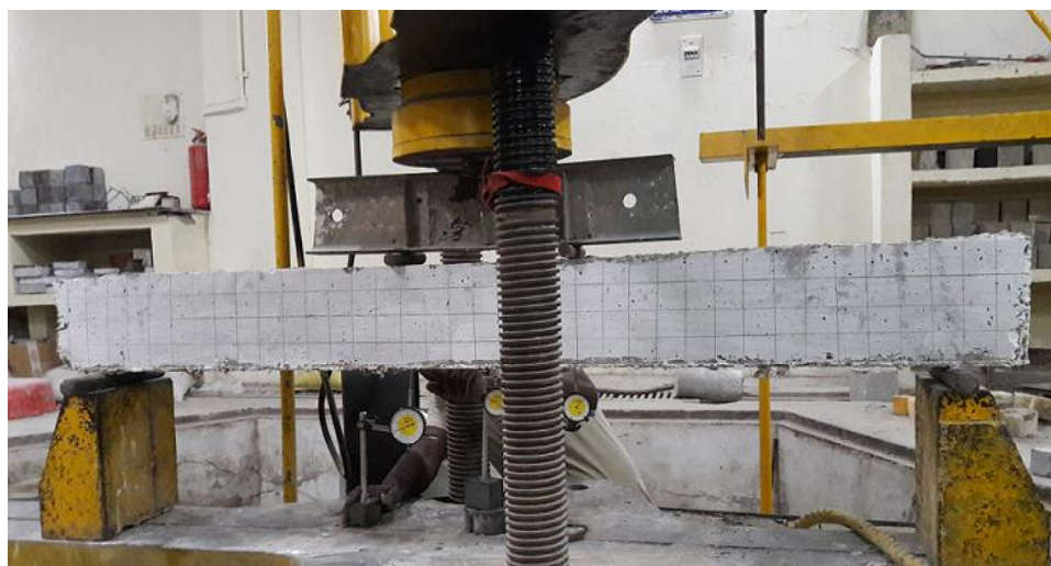
Figure 4.17b Testing of RC beam under flexure
