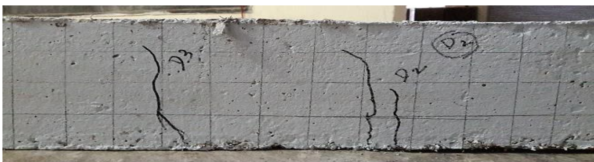
5.8 (b) SFRC beam after complete failure
