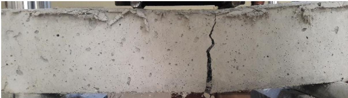
Figure 5.5 Flexural failure of PPFRC specimen
