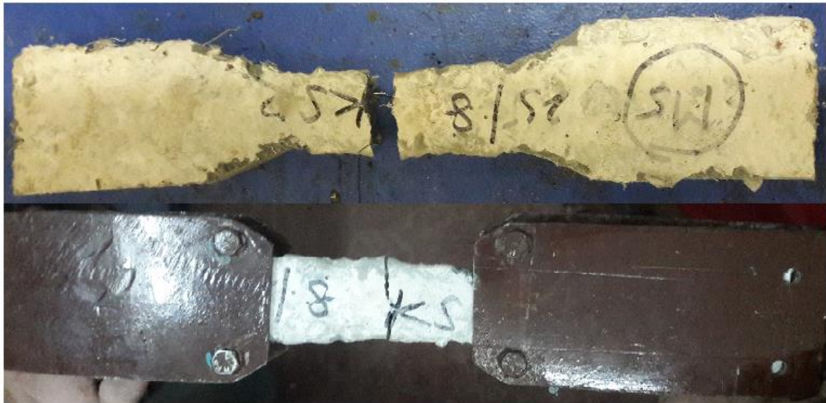
Figure 6.5 Failure patterns of dog-bone specimens of ECC
