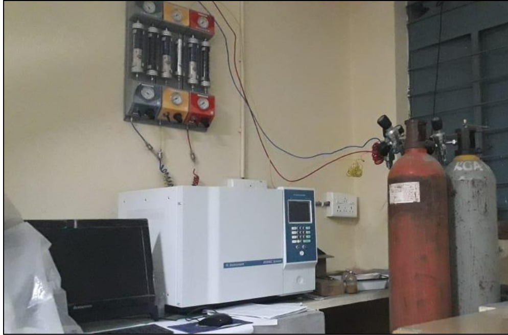
Fig. 3.4 Gas Chromatography system for biogas analysis
