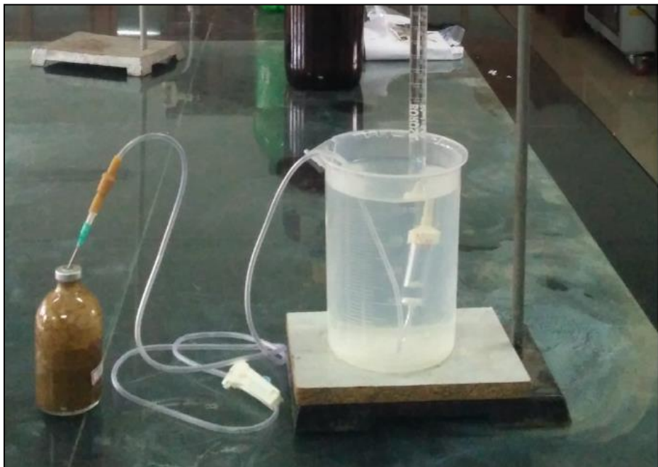
Fig. 3.3 Biogas measurement by the downward water displacement method
