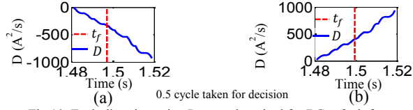
Fig 10. Fault direction using Proposed method for BC-g fault for scenario 2 a) R_1 b) R_2 .
