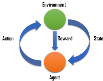
Fig. 2. Reinforcement Learning Architecture
