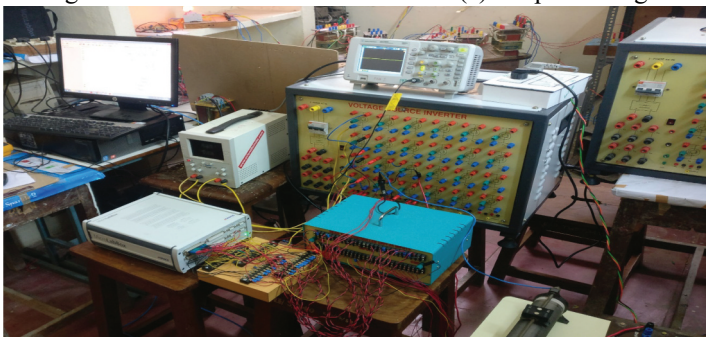
(d) Experimental set up of single-phase nine-level cascaded T-type RSC-MLI
