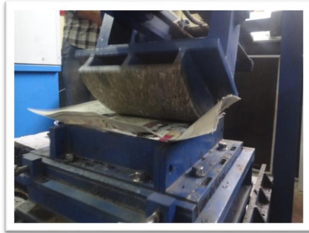
Fig. 3.11 Segmented steel-wheeled roller compactor
