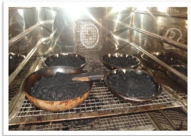
Fig. 3.10 Short-term aging of bituminous mixtures
