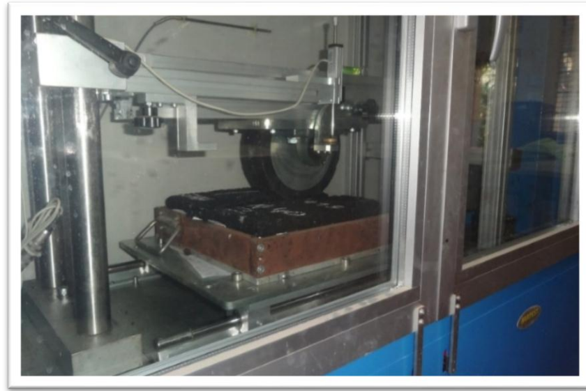
Fig. 5.2 Slab sample being tested in the wheel tracking machine
