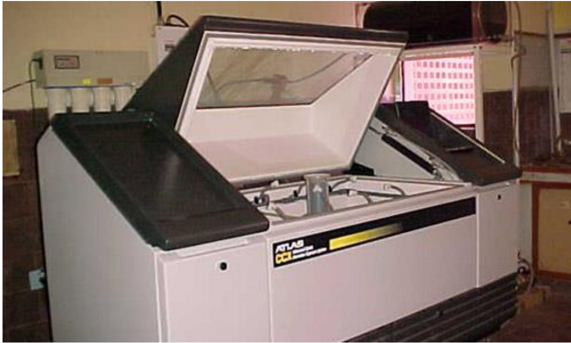
Fig. 2.7. Photograph of salt spray test chamber
