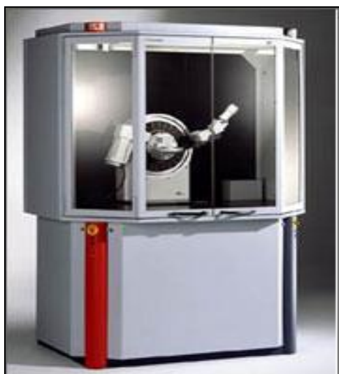
Fig. 2.3. X-ray diffractometer - Bruker AXS D8 Advance
