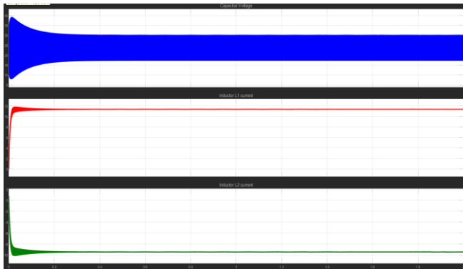
Fig. 11. Capacitor Voltage, Inductor L_1 current and L_2 Current
