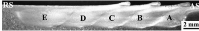
Fig. 2.6. Low-magnification image of 5-pass overlapping FSP [Xue et al., (2013)].
