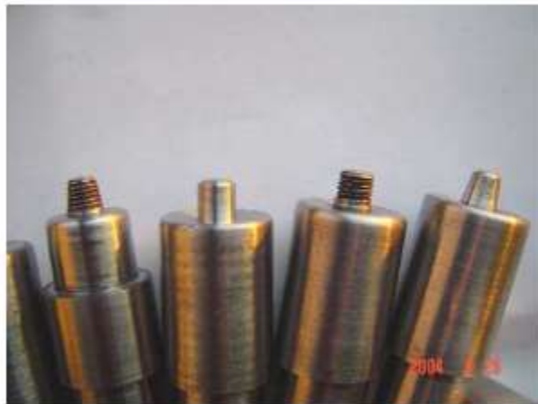
Fig. 2.4. FSW tools with different pin profiles [Zhao et al., (2005)].
