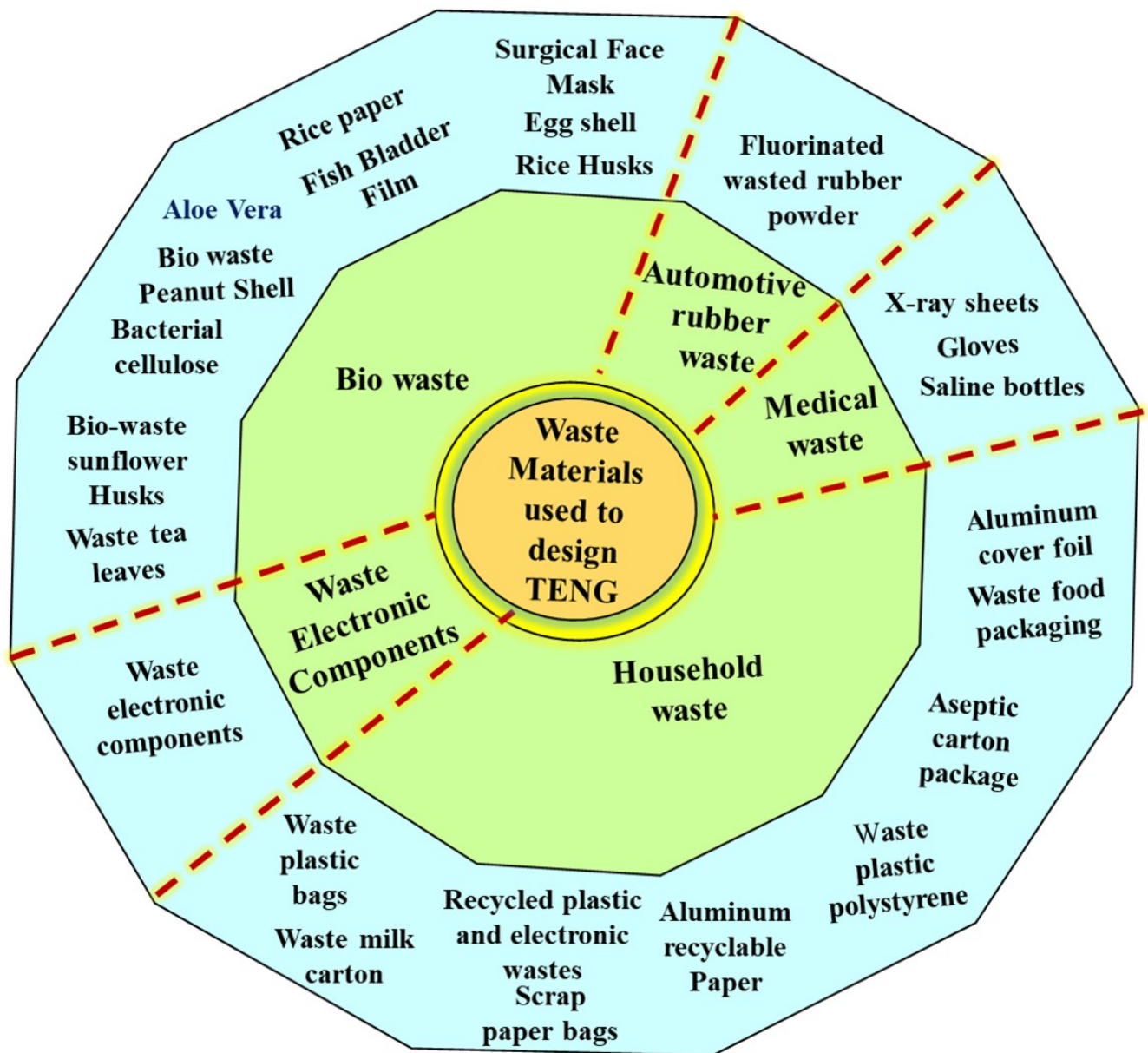
Figure 3.4: Waste materials used in TENG. Adapted from [43]
