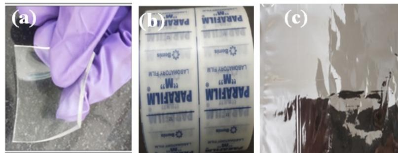
Figure 3.7: Basic Materials (a) PDMS (b) Laboratory parafilm (c) Aluminium foil.
