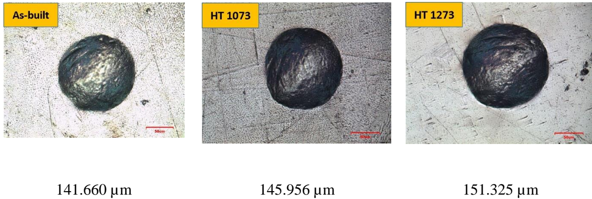
Figure 6.6 Typical indentation of SS 316 samples during ABI test
