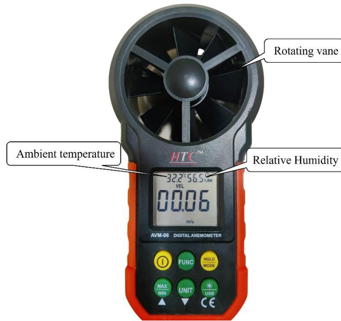
Figure 3.5 Anemometer with its distinct components and respective functions
