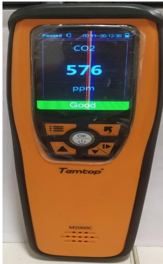
Figure 4.12 Air quality detector used to measure concentrations of CO 2 , PM 2.5 and PM 10 .
