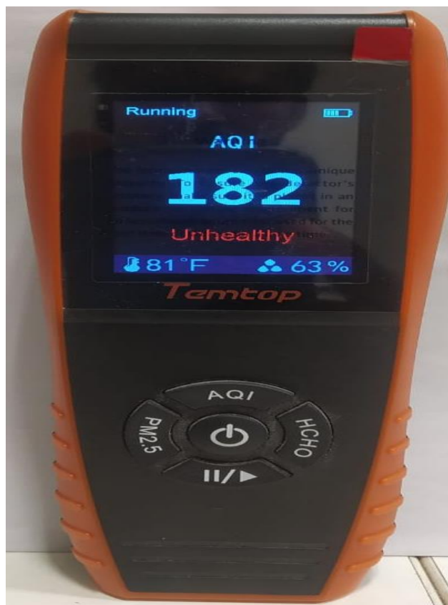
Figure 4.13 Laser particle multi-functional detector used to measure AQI
