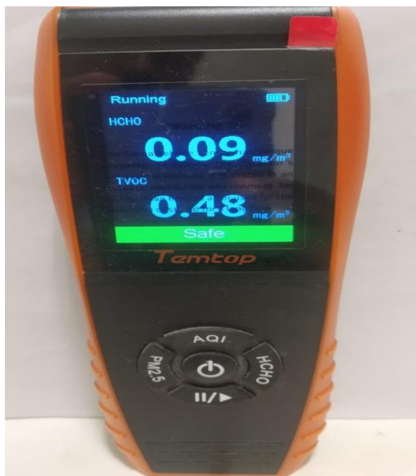
Figure 4.11 Laser-particle multi-functional detector used to measure HCHO and TVOC concentrations
