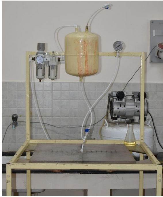
Figure 3. 2 Experimental Setup for Reinforcement Mat Permeability Measurement
