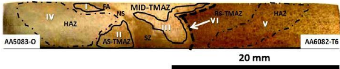
Figure 2.14: Optical picture of FSWed AA5083-AA6082 after a 7-day immersion test in 3.5 percent NaCl solution [Donatus et al., (2015)].
