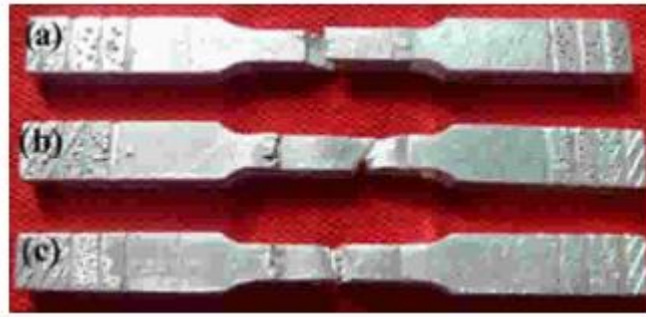
Figure 2.7: Failure regions of dissimilar FS welded joints at (a) 36 mm/min, (b) 63 mm/min and (c) 60 mm/min [Palanivel et al., (2014)].
