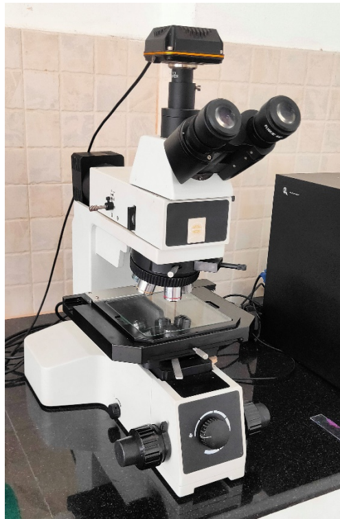
Fig 3.7: Optical microscope used for examination of microstructure
