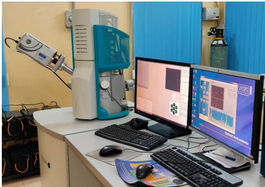
Fig 3.9: SEM used for examination of microstructure
