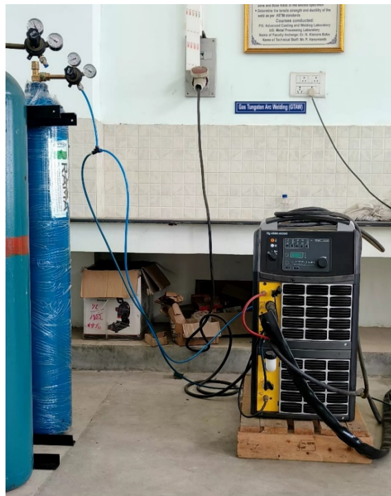
Fig 3.2: Power source used in GTA welding
