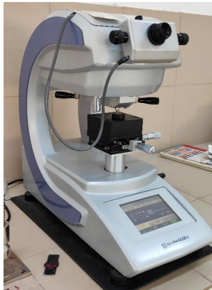
Fig 3.10: Vickers micro hardness for testing of samples
