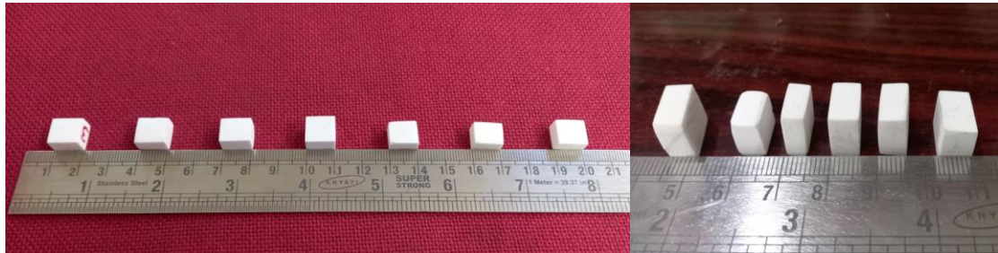
Fig.4.21: Samples prepared for sliding wear test
