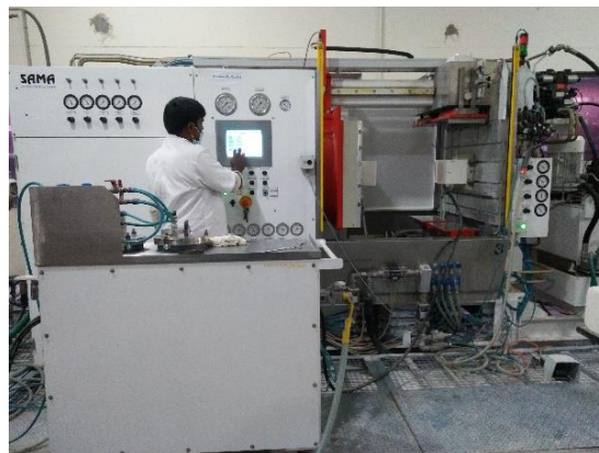
Fig.3.12: Pressure Slip Casting Machine in operating condition (PCM-100, SAMA, GmbH, Germany).
