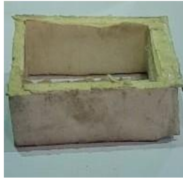
Fig.3.11: Non-Permeable rubber- mould used for cold iso-static pressing
