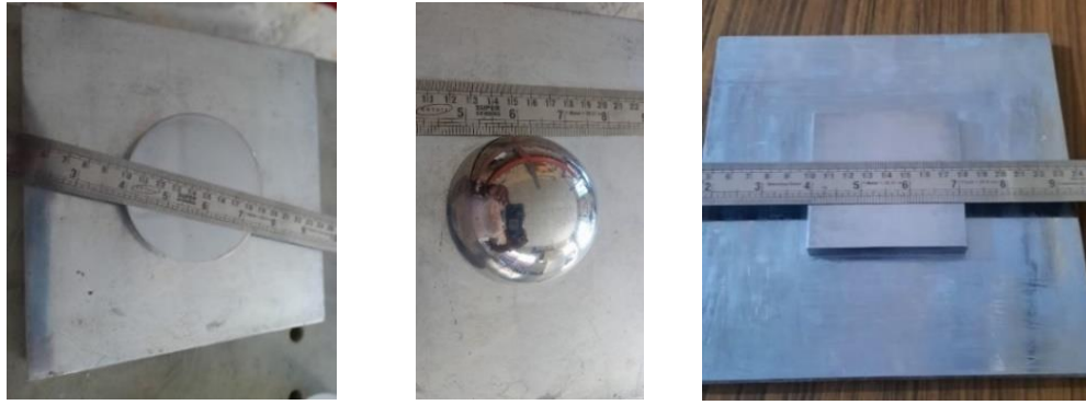
Fig. 3.5: Patterns made for cast of a) Cylindrical disc b) Spherical ball c) Square patterns
