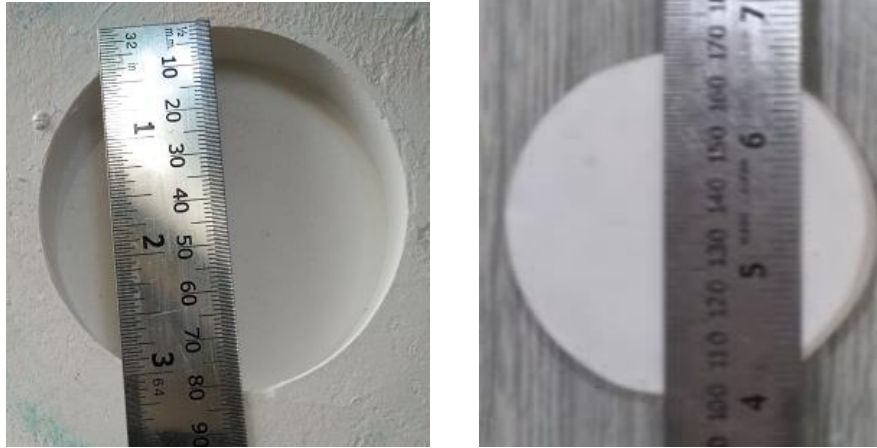
Fig.4.32: Aluminum Titanate cylindrical discs by Conventional Slip Casting.
