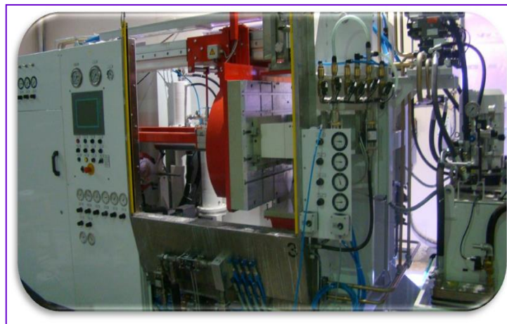
Fig.1.9: Pressure Slip Casting Machine (PCM) -100-N (SAMA GmbH) at ARCI
