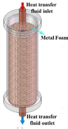
Fig 2.3 Shell and tube heat exchanger with metal foam [98]
