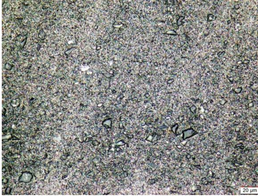
Fig. 4.4. SZ of Al6082-T6/SiC with 6 vol.% of reinforcement
