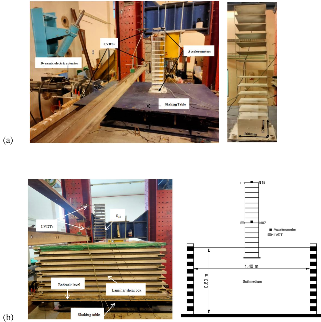
Figure 3.15 Installation steps implemented for a 15-storey building with two subterranean levels on the shaking table: (a) fixed base, and (b) flexible base (Hoseny et al., 2023).
