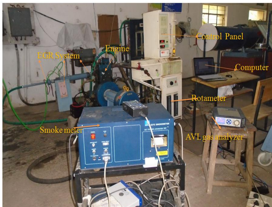
Fig. 3.1. Engine experimental set-up of the VCR engine test rig.
