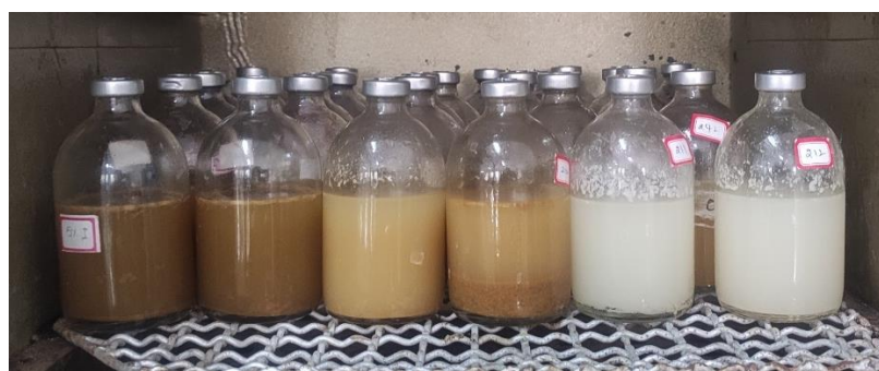
Figure 3. 5 Biochemical methane potential experimental set-up
