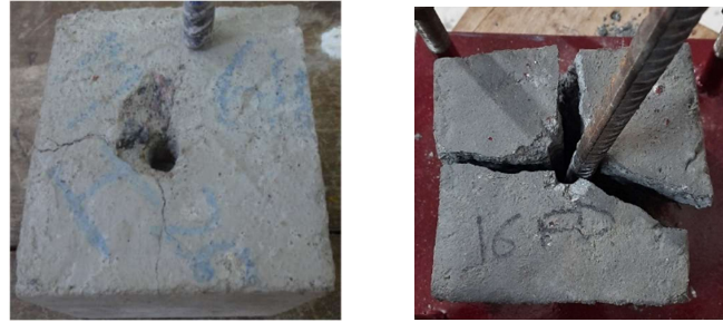
Figure 5.20: a) Pullout failure b) splitting failure
