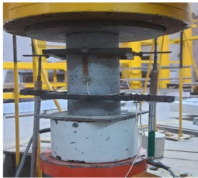
Figure 3.11: Test setup for Young's modulus and stress-strain curve
