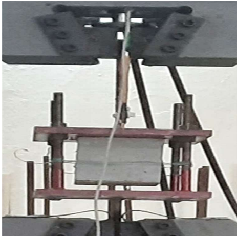
Figure 5.1: A) experimental test setup B) force distribution in pullout specimen-a) 2.5D b) 5D c) Full depth of the specimen
