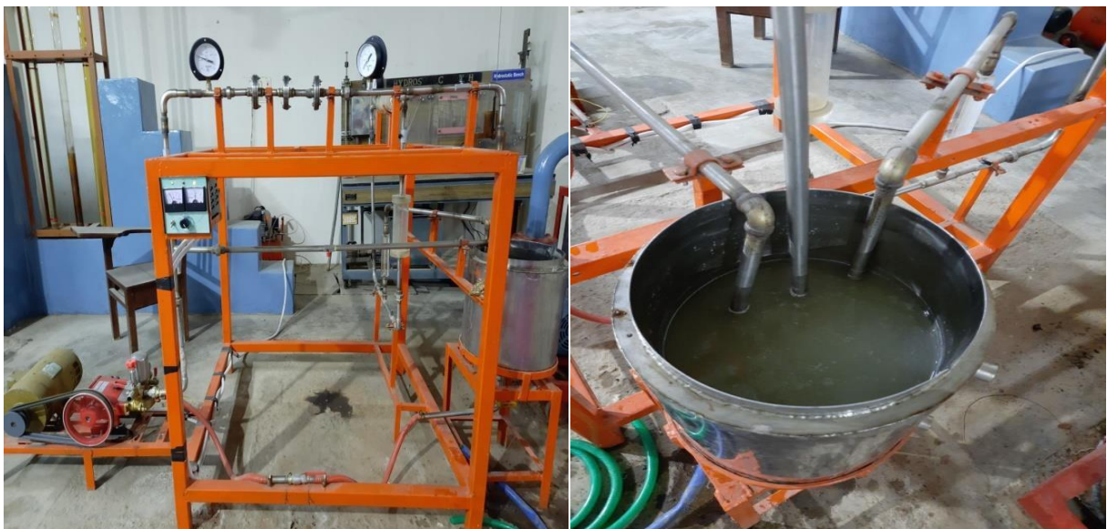
Figure 3.4 Fabricated Hydrodynamic cavitation set-up
