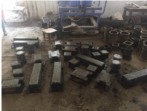
Figure 4.7 Cast specimens of alccofine-1203 based concrete mixes
