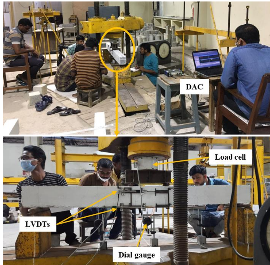
Figure 6.8 Experimental testing of BFRP-reinforced concrete beams
