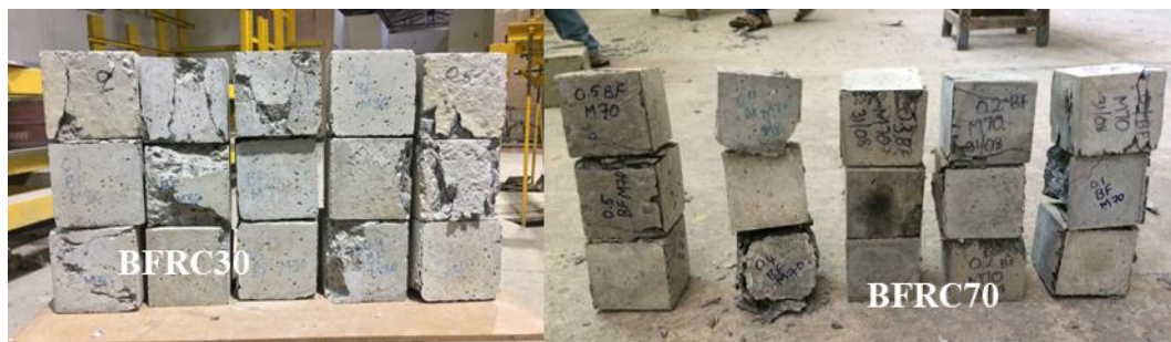
Figure 5.23 Failure of compressive strength specimens of BFRCs
