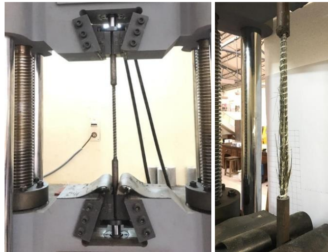
Figure 6.6 Tensile test on BFRP rebar
