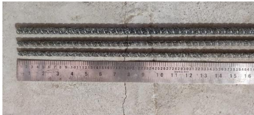
Figure 6.1 Helical wound sand coated BFRP rebars
