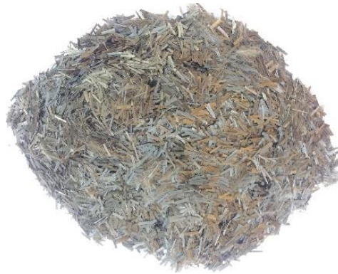
Figure 5.19 Chopped basalt fibers
