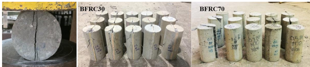
Figure 5.28 Failure of split tensile strength specimens of BFRCs
