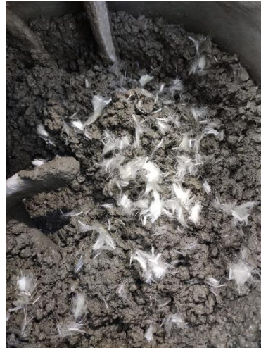
Figure 5.2 PVA fibers mixing into wet concrete
