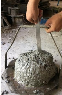
Figure 4.8 Slump cone test on alccofine-1203 based concrete mix
