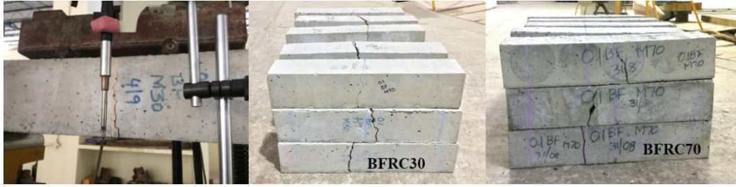
Figure 5.26 Failure of flexural strength specimens of BFRCs
