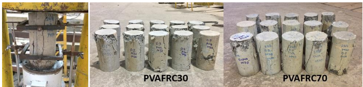
Figure 5.13 Failure of PVAFRCs specimens under the test of uniaxial compressive stress-strain behaviour
