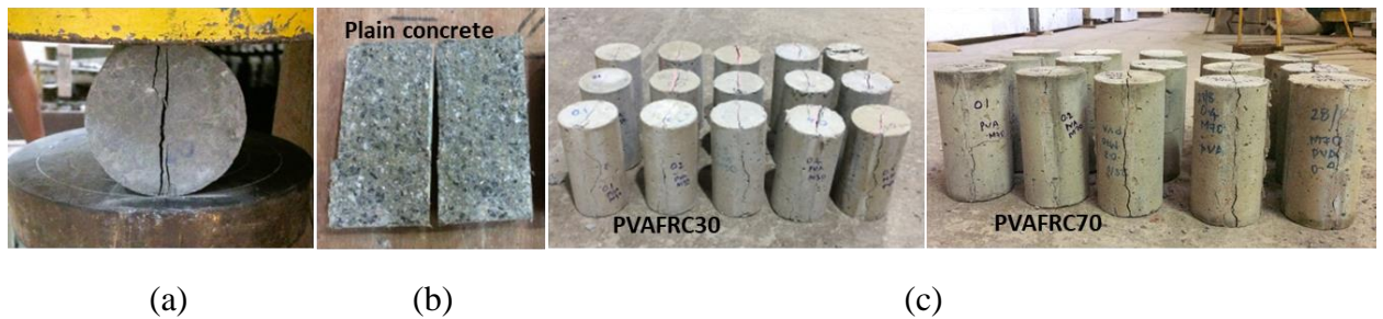
Figure 5.11 Failure of split tensile strength specimens: (a) crack at ultimate load, (b) plain concrete, (c) PVAFRC
