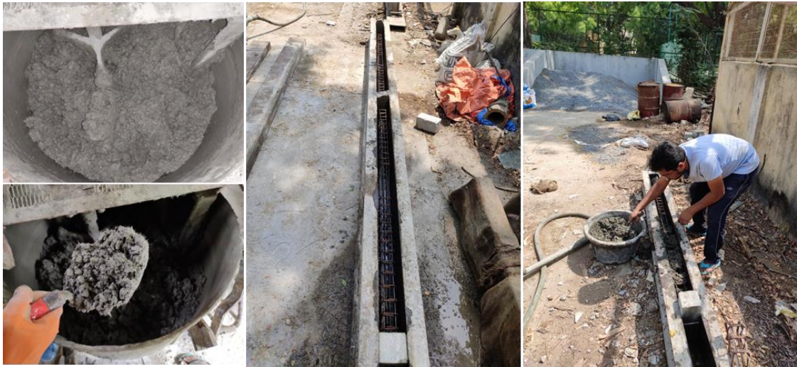
Figure 6.7 Cast of BFRP-reinforced concrete beams
