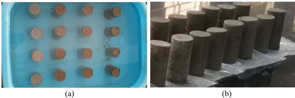
Fig. 3.8. Treated specimens subjected to wetting-drying cycles (a) during wetting (b) before oven drying
