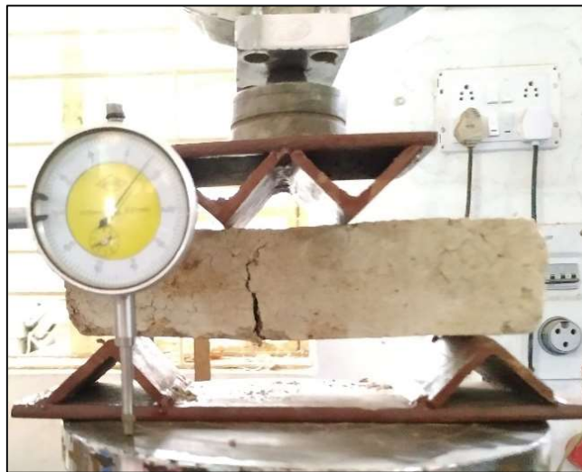
Fig. 4.13. Failure of flexural strength beam specimen
