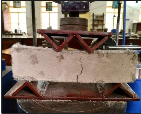
Fig. 4.37. Failure of fiber reinforced soil-geopolymer beam specimen under flexure
