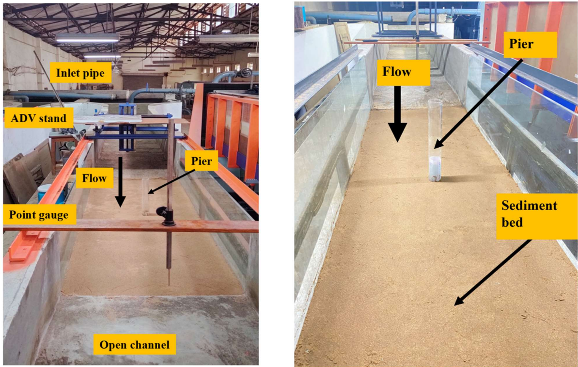
Figure 3.1: Photographic view of the working section of the flume used in experiments.
