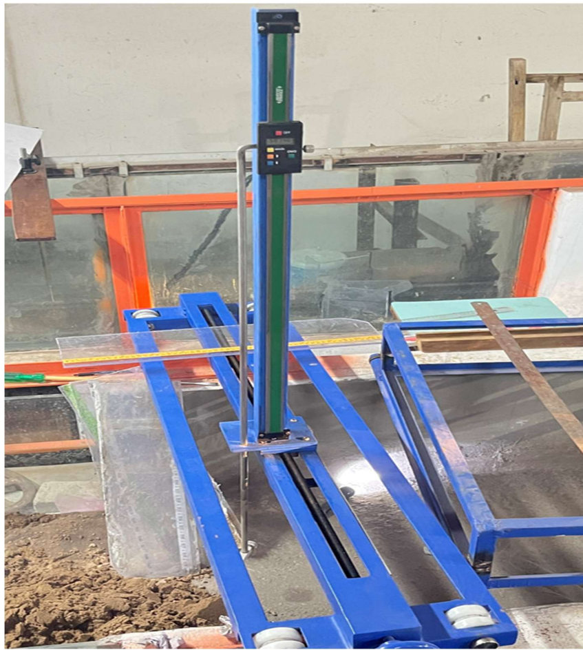
Figure 3.8: Photographic view of digital point gauge.
