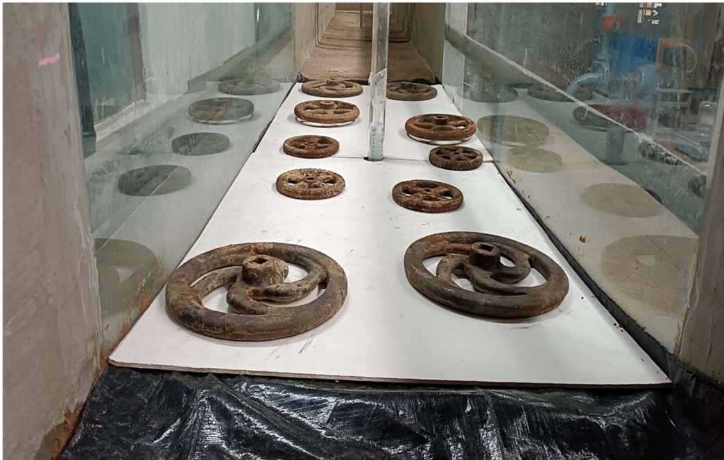
Figure 3.10: Covering sediment bed with PVC sheet and plywood.
