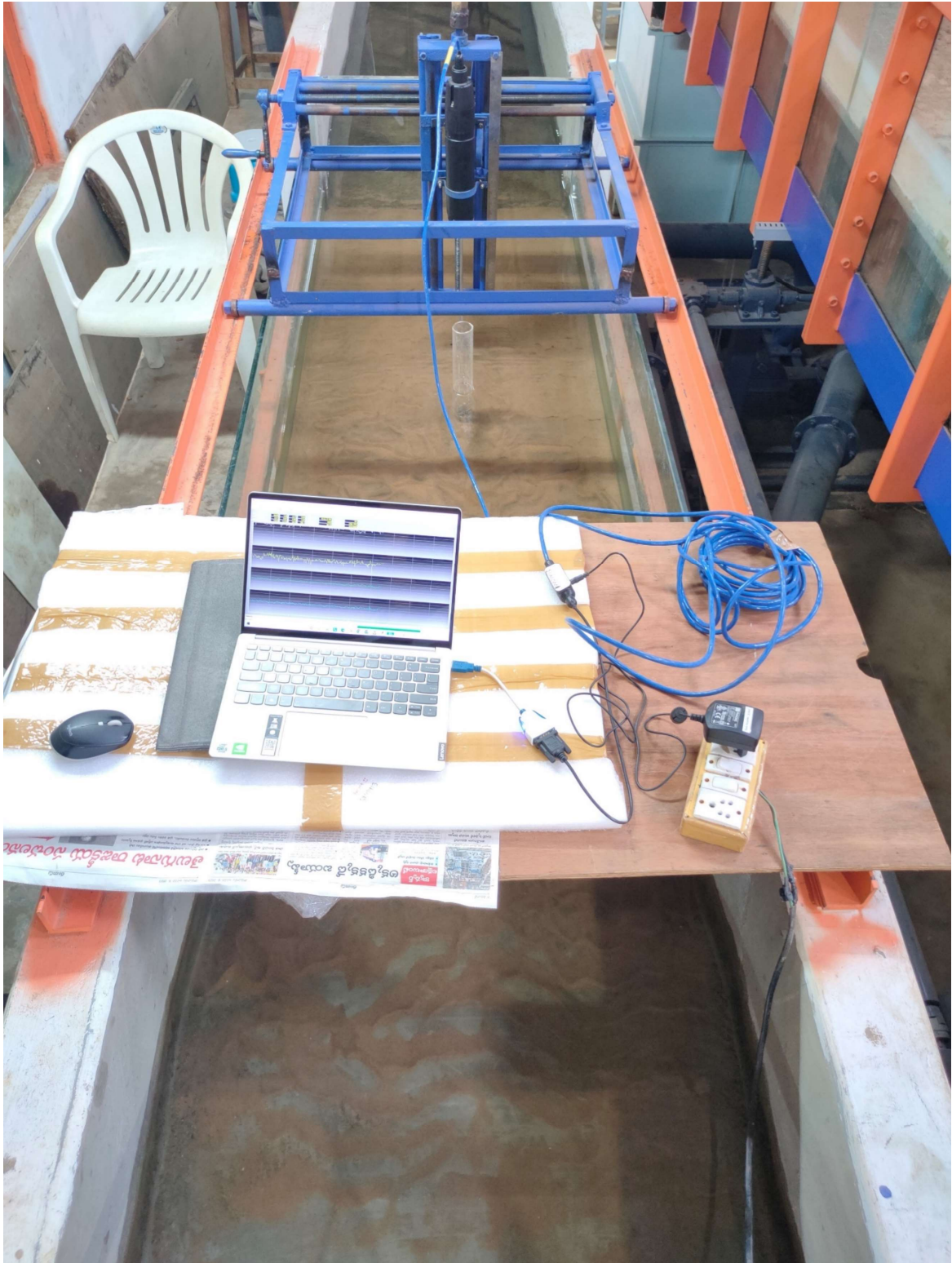
Figure 3.7: Photographic view of an ADV instrument setup.
