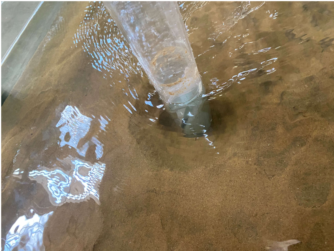
Figure 3.11: Scour around the pier without collar after four hours of elapsed time
