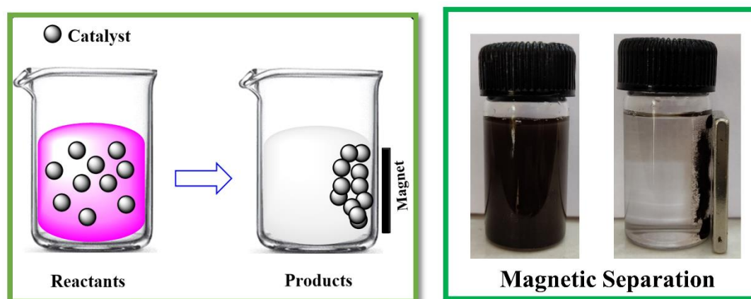
Figure 1.1. Schematic of magnetic separation of the catalyst
