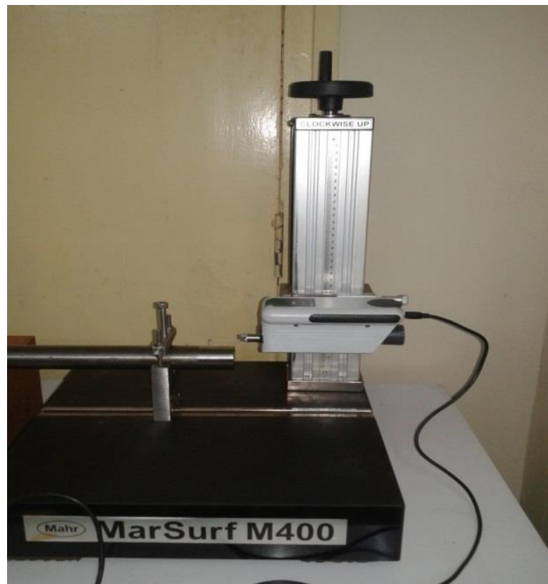
Figure 4.8: Surface roughness measurement using MarSurf
