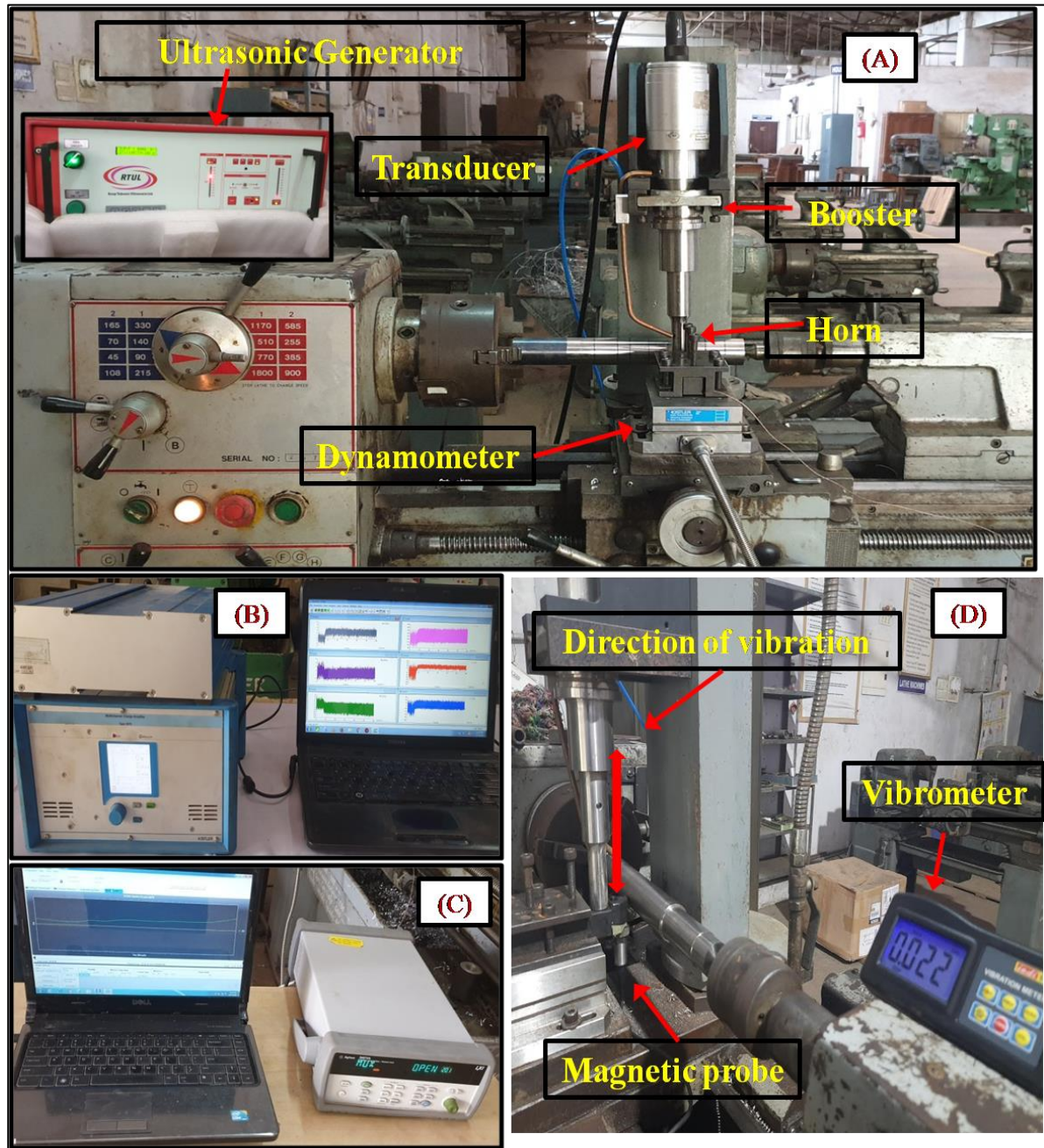
Figure 4.4: Experimental setup and measuring system used for UVAT process
