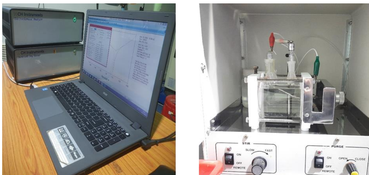
Fig. 2.17. CH instrument electrochemical workstation along with the electrochemical cell
