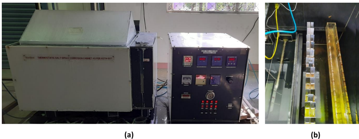
Fig. 2.19. (a) Salt spray cabinet and (b) sample holder containing the mild steel substrates for corrosion test
