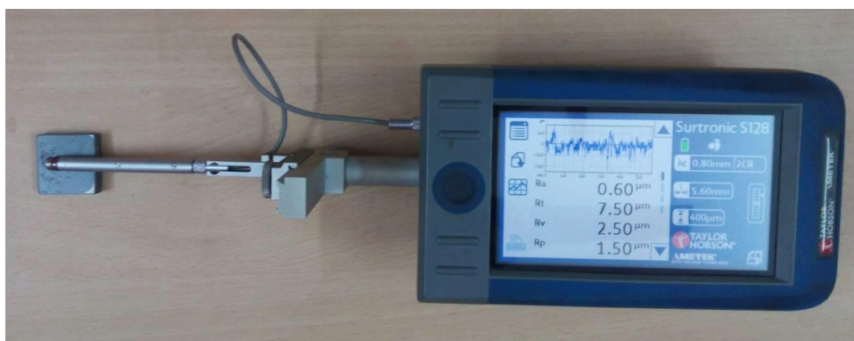
Fig. 3.4 Surface Roughness Tester Surtronic S-100 (Taylor Hobson)
