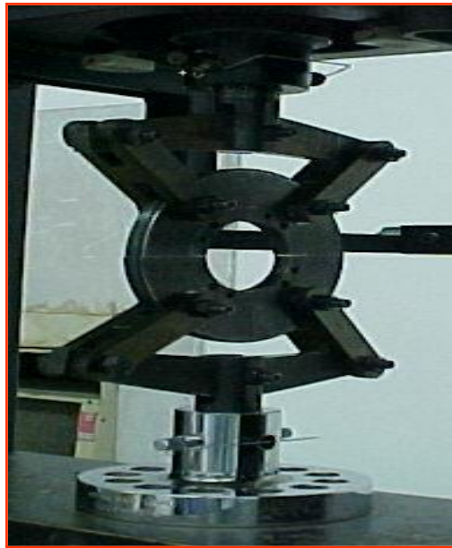
Figure 3.19: Carbon-Epoxy ring specimen testing using split disc fixture
