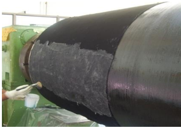
Figure 6.2: Hand lay-up of Impregnated Panox Fabric
