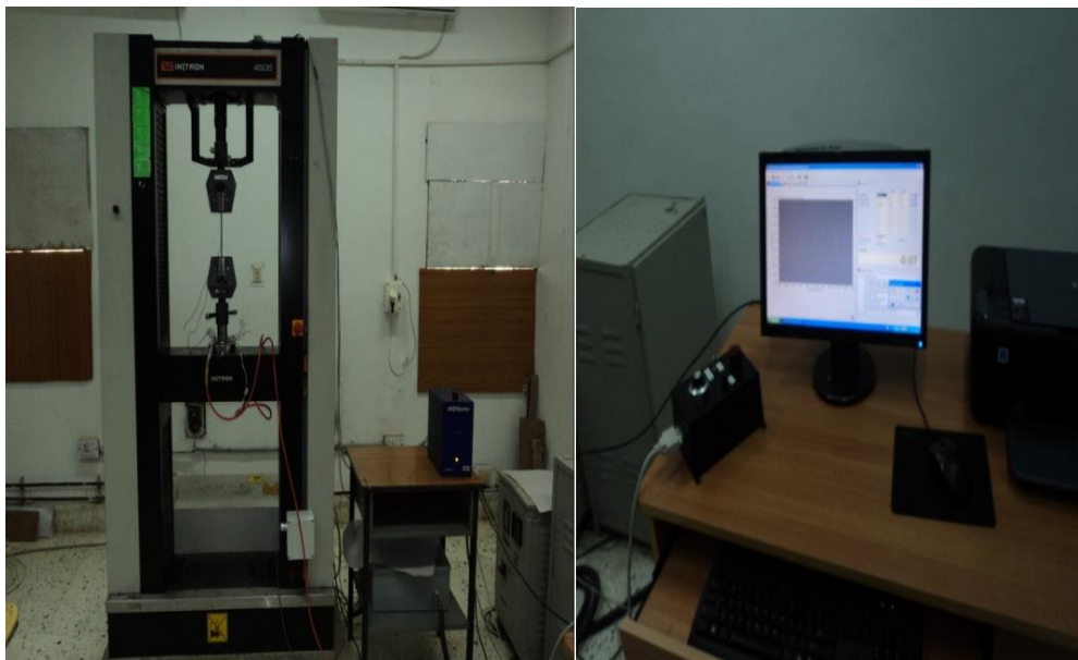
Figure 3.7: Mechanical Test Set Up (Instron with specimen & Data acquisition system)
