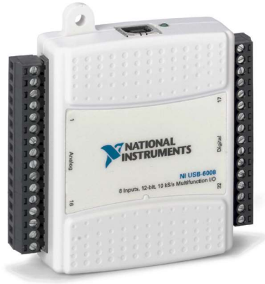
Figure 5.20 NI USB-6008 DAQ
