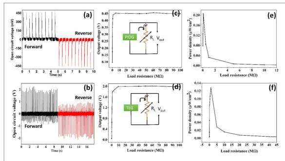
$\textbf{Figure 4.} Forward and reverse connection V_{oc} of (a) PIOG, (b) TEG; output voltage of (c) PIOG, (d) TEG across the different load across the$ resistances; instantaneous power density of (e) PIOG, (f) TEG across the different load resistances.
