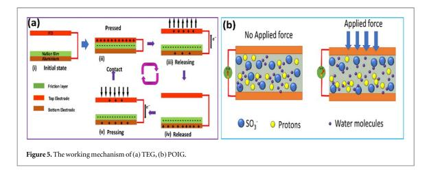
characteristics of PIOG, and TEG is in good agreement with the previously reported literature [61, 62]. The maximum instantaneous output power density of  $\sim 0.205 \,\mu\text{W cm}^{-2}$ ,  $0.128 \,\mu\text{W cm}^{-2}$  at load resistance values of  $\sim$ 100 K $\Omega$ , 1 M $\Omega$  for PIOG and TEG, respectively.
