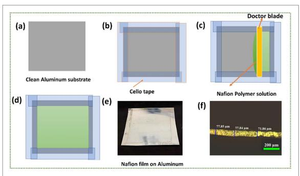
**Figure 1.** (a)—(d) schematic of the steps involved in the Nafion film preparation, (e) Obtained Nafion film on the aluminum substrate, (f) cross-sectional view of the Nafion film in the optical microscope for thickness measurement.
