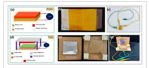
**Figure 2.** (a) 3D Schematic of PIOG device, (b)–(c) photographs of the fabricated PIOG device, (d) 3D Schematic of TEG device, (e)–(g) photographs of the TEG device fabrication steps and final device.
