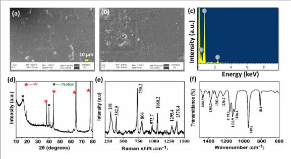
Figure 3. (a)—(b) SEM image of the Nafion film surface, (c) EDX spectrum collected from the Nafion surface, Nafion film (d) XRD pattern, (e) Raman spectrum, and (f) FT-IR spectrum.
