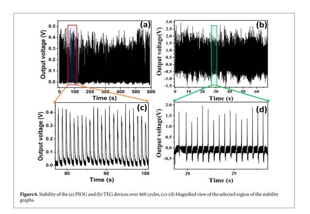
zero potential across the electrodes. When force is applied to the POIG device, the potential difference is generated due to the redistribution of protons and sulfonic ions in the Nafion film, as shown in figure 5(b). Furthermore, the stability of the nanogenerator was tested over 460 cycles, and responses are shown in figures 6(a)–(b). Figures 6(c)–(d) represent the magnified views of the selected regions of the stability graphs. The high stability of PIOG, and TEG can be evidenced in figure 6.
