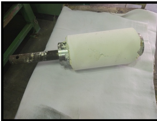
Fig. 3.9 Mandrel (PoP cast over a steel rod)
