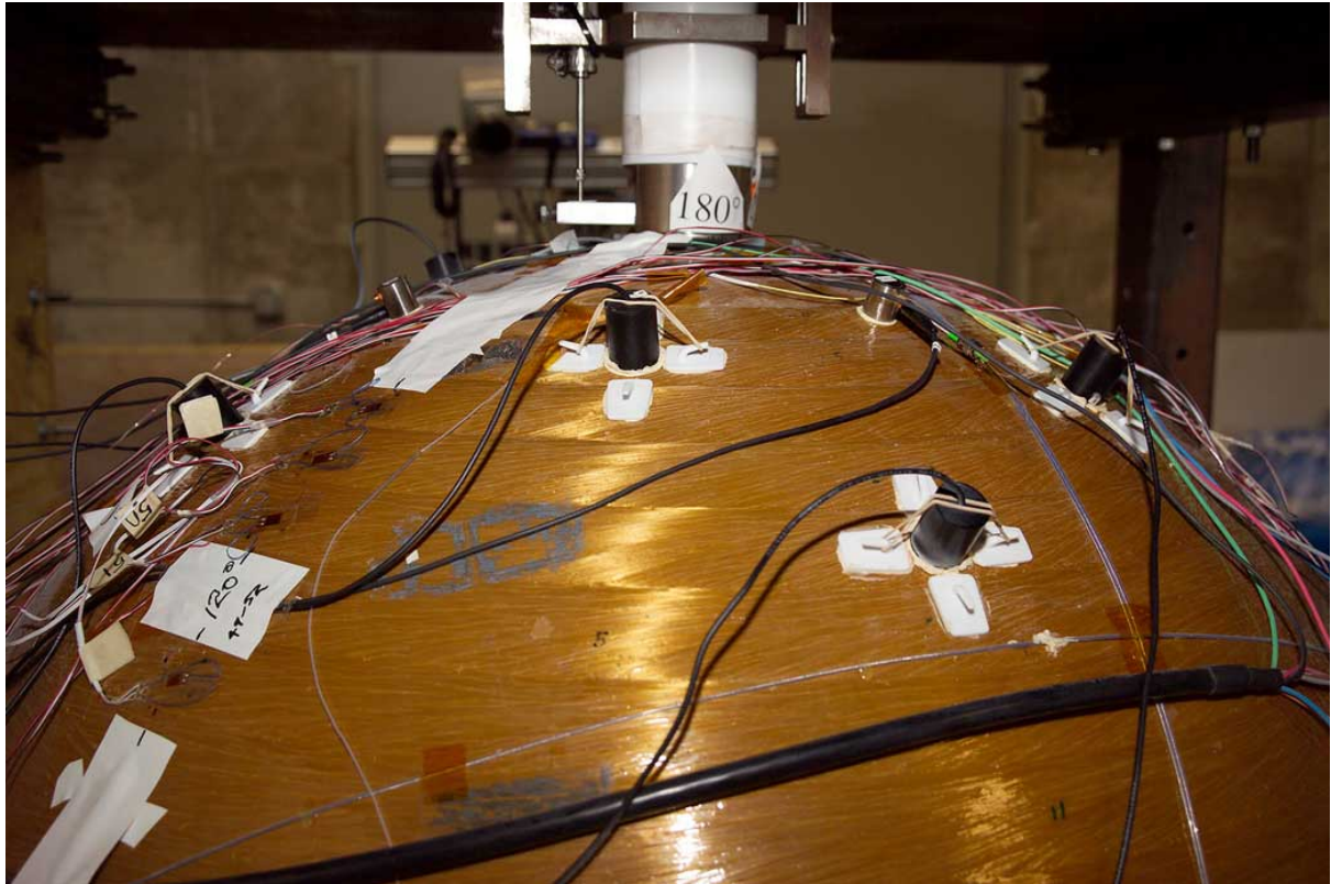
Fig. 1.8 Acoustic Emission Testing of a composite pressure vessel (Source: Grand Research Store)
