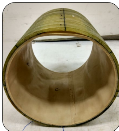
Fig. 5.1 Cylindrical GFRP composite sample with rubber lining
