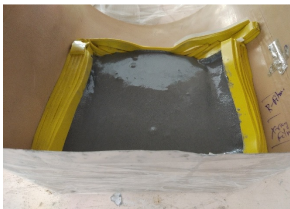
Fig. 5.2 Cylindrical GFRP composite sample with propellant adhesively bonded to rubber
