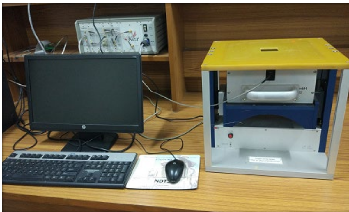
Fig. 3.14 Single sided low field NMR system (A: Spectrometer, B: MOUSE with HP lift)
