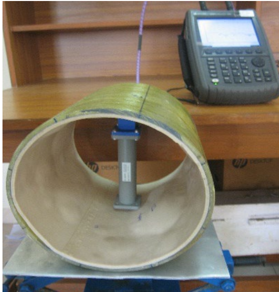
Fig. 5.12 Microwave NDE inspection system for composite structures using single sided open ended wave guide method.
