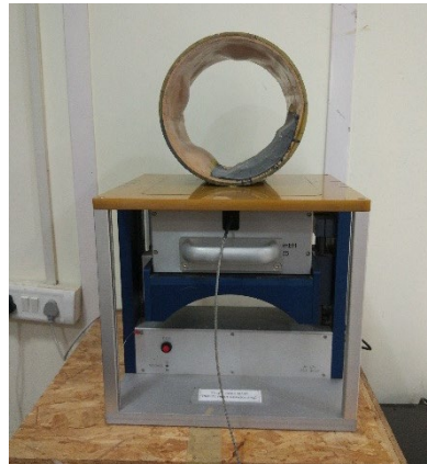
Fig. 5.4 Stepper motor assembly for performing profile NMR experiments
