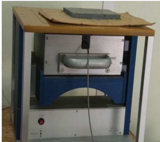
Fig. 6.1 Profile NMR-MOUSE (PM 25)
