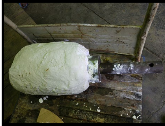
Fig. 3.9 Mandrel (PoP cast over a steel rod)
