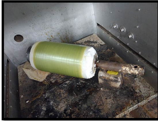
Fig. 3.12 Wound mandrel in curing oven
