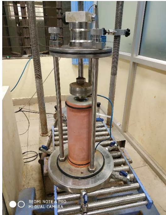
Fig. 5.1 Setup used in RLT test
