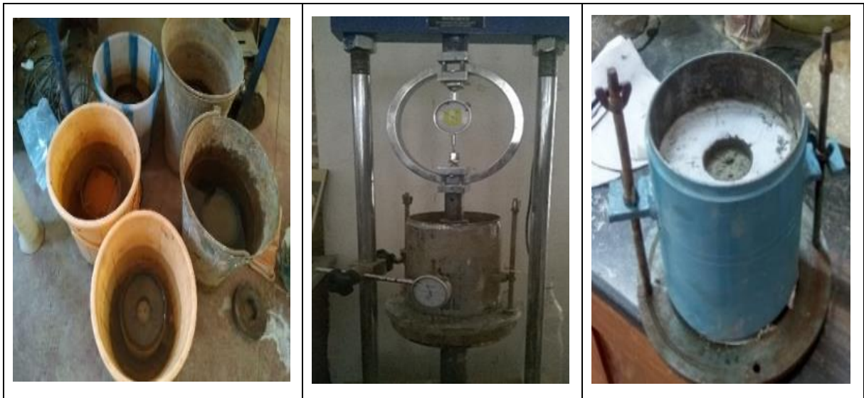
Fig. 4.8. CBR test of pond ash specimens
