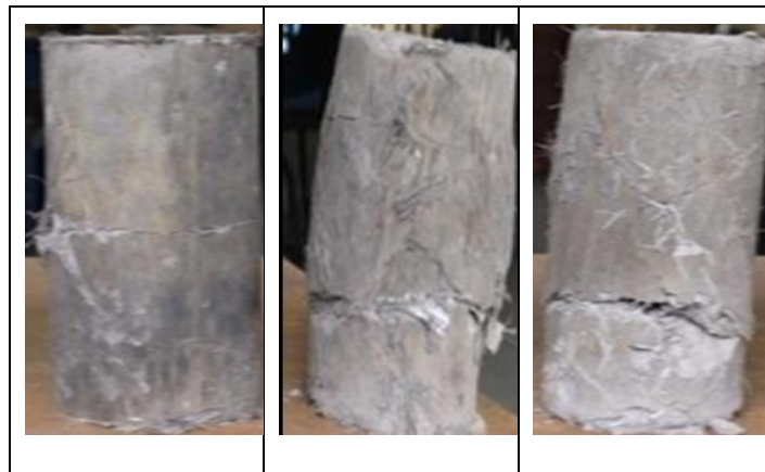
Fig. 4.14. Failure specimens of PLF mixes
