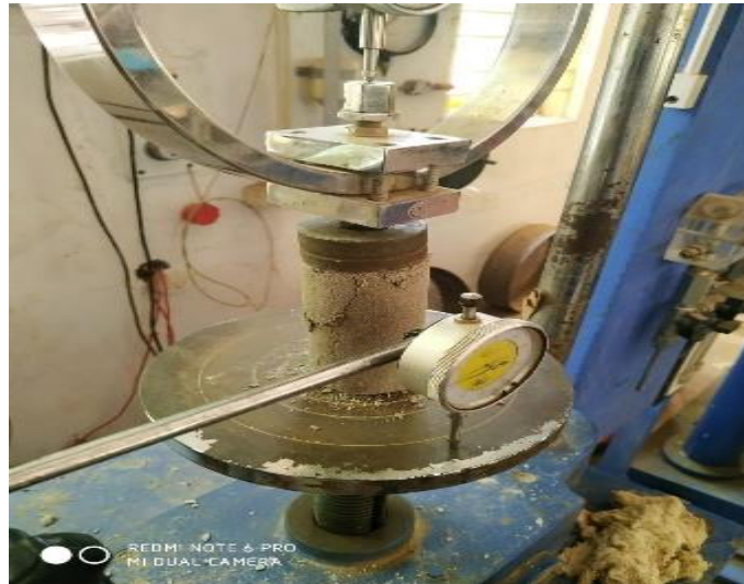
Fig. 4.7. UCS sample during the test
