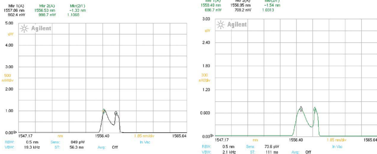
Figure 5 Spectral response of the Bragg reflected peak at different temperatures: (a) 145^\circ\text{C} and (b) 185^\circ\text{C} . [Color figure can be viewed in the online issue, which is available at wileyonlinelibrary.com ]
