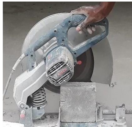
(b) Cutting of the wedge splitting test using concrete cutter
