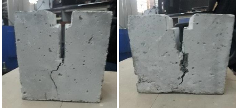
Figure 4.40. Failure pattern of specimens without guide notch
