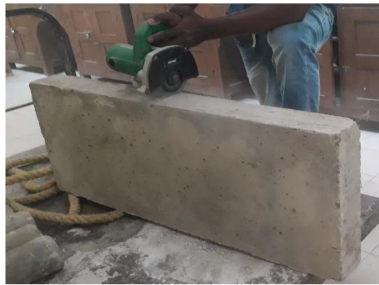
Figure 4.8. Notch cutting of beam specimen
