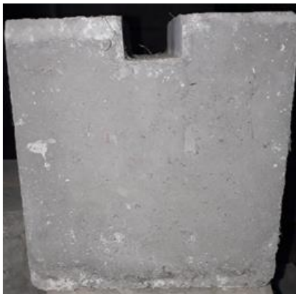
(a) Specimen with cast groove
