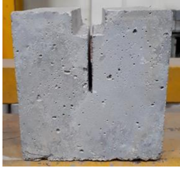
(c) Without guide notch specimen
