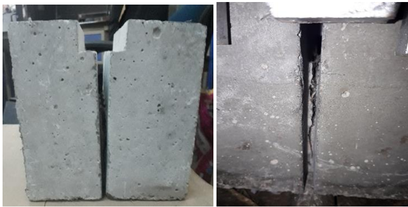
Figure 4.41. Failure pattern of specimens with guide notch
