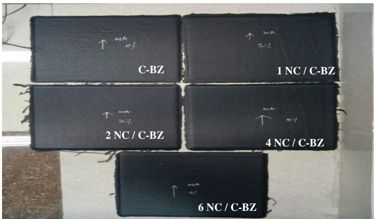
Figure 5.7 Blank carbon fiber - benzoxazine resin composite and 1, 2, 4, 6 wt% nanoclay added carbon fiber - benzoxazine resin composites
