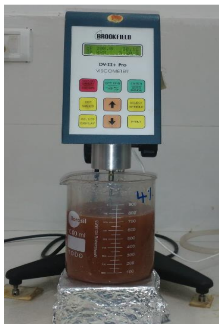
Figure 4.4 Measurement of viscosity of 4 wt% nanoclay filled CE resin by Brookfield viscometer.
