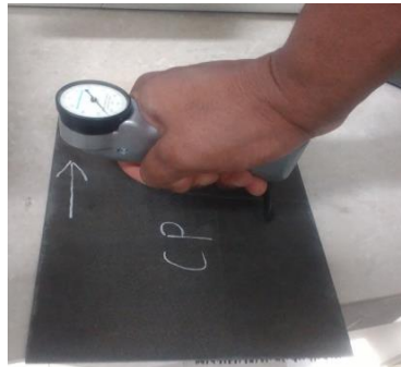
Figure 3.10. Measurement of hardness on carbon fiber – phenolic resin composite
