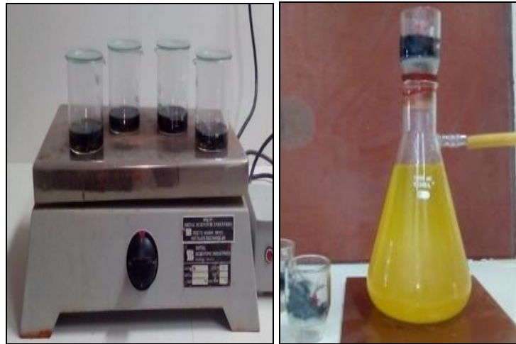
Figure. 3.9. Resin content test by acid digestion
