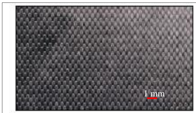
Figure 4.2 PAN based woven carbon fabric
