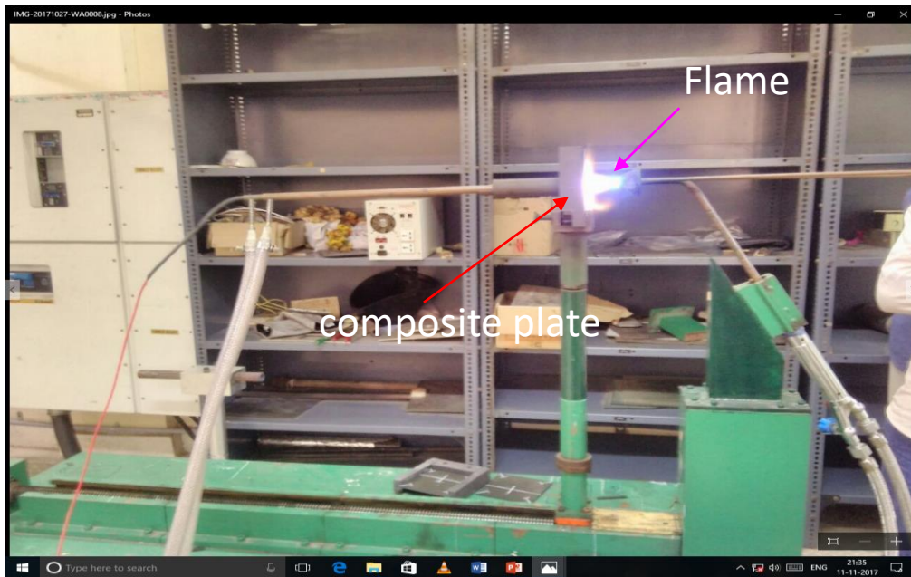
Figure 4.18. Oxy-acetylene torch test of type -II composite at heat flux 125 \text{ W/cm}^2
