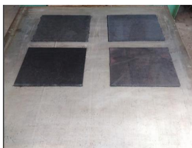
Hand Lay - up of composites ( 12 Layers ,Size : 300 x300 mm)
