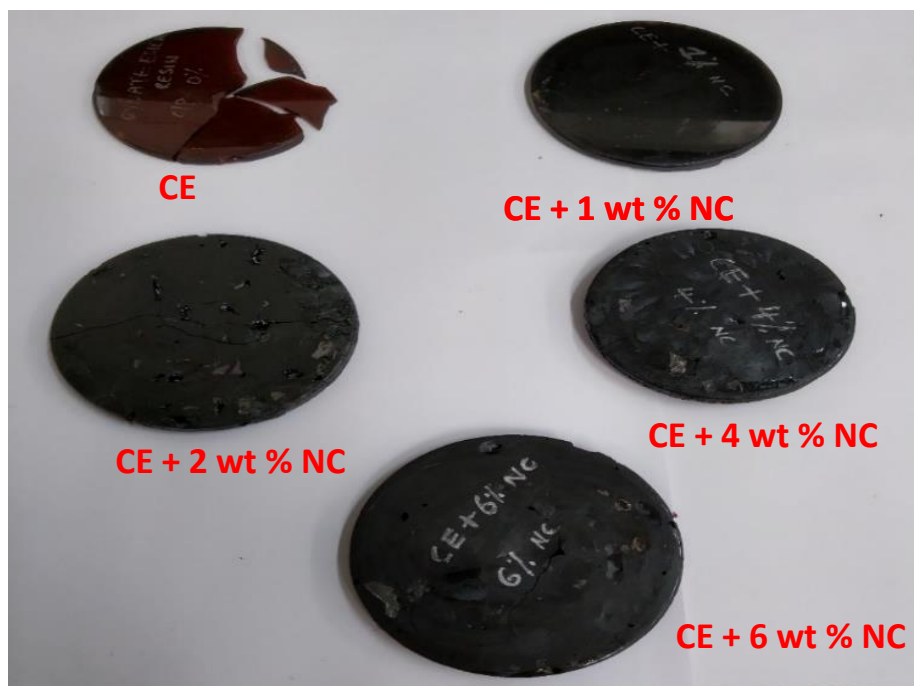
Figure 4.5 Cured cyanate ester resin and cyanate ester resin - nanoclay composites
