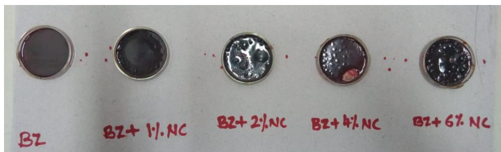
Figure 5.4 Cured blank BZ resin and 1, 2, 4, 6 wt% nanoclay filled BZ resin composites
