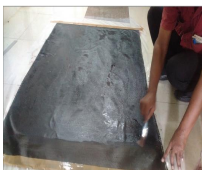
Hand impregnation of carbon cloth (fabric) with clay filled benzoxazine resin
