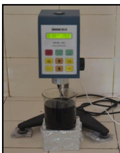
Figure 3.5. Measurement of viscosity of resin by Brookfield viscometer
