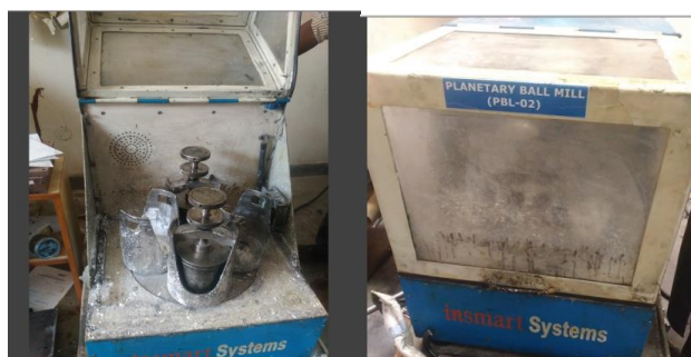
Ball Milling of Clay and Phenolic resin
